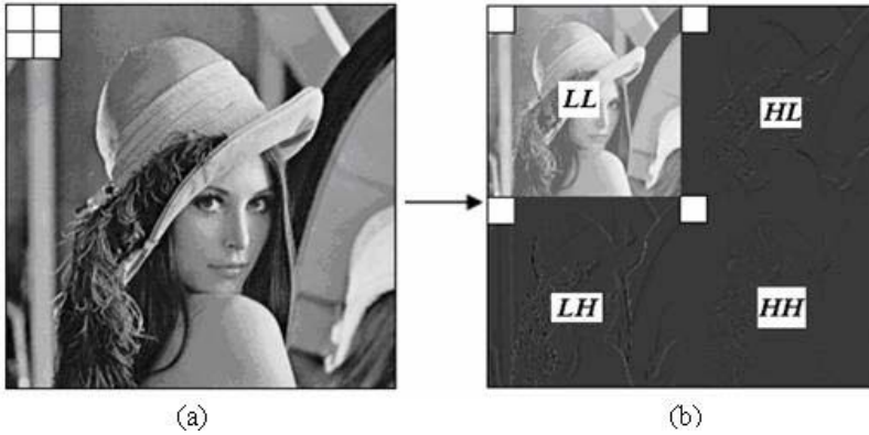
Fig. 1. The mapping between spatial block and DWT coefficients (a) "Lena" image, (b) the one-level DWT of "Lena"
