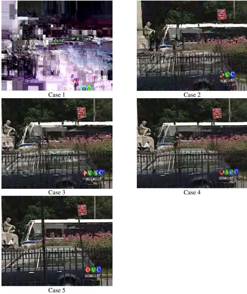
Fig. 9. Visual patterns of decoded video for the given bitstream with access key of corresponding access right
